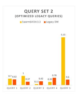
A healthcare company compared Swarm64 DA-accelerated PostgreSQL performance to that of their Netezza data warehouse. The test involved 10TB of data. Swarm64 DA accelerated free, open source PostgreSQL 11 on a single server equipped with an FPGA.
